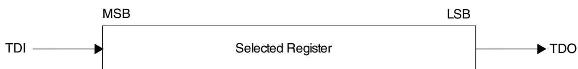
Figure 52-3. Shifting data through a register
