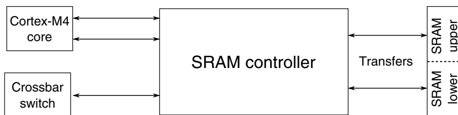
Figure 3-24. SRAM controller configuration
