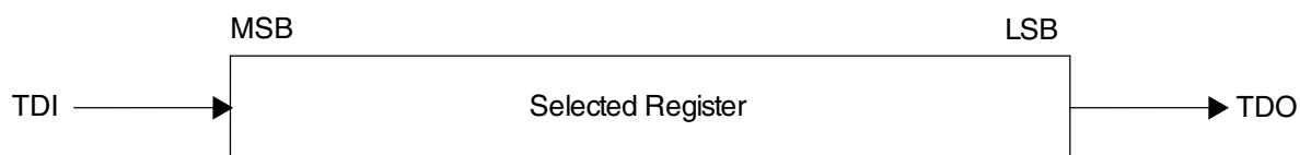
Figure 49-3. Shifting data through a register
