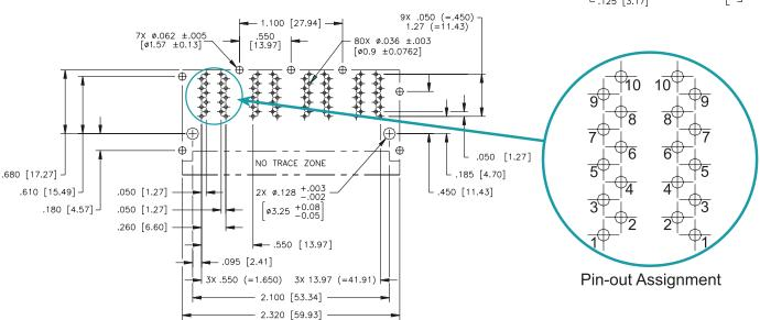
SUGGESTED PC BOARD LAYOUT VIEWED FROM COMPONENT SIDE UNLESS OTHERWISE SPECIFIED DIMENSIONAL TOLERANCE IS  $\pm .002$
