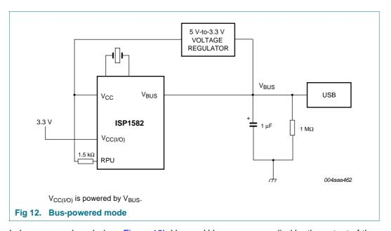
In bus-powered mode (see Figure 12),  $V_{CC}$  and  $V_{CC(I/O)}$  are supplied by the output of the 5 V-to-3.3 V voltage regulator. The input to the regulator is from  $V_{BUS}$ . On plugging the USB cable, the ISP1582 goes through the power-on reset cycle. In this mode, OTG is disabled.
