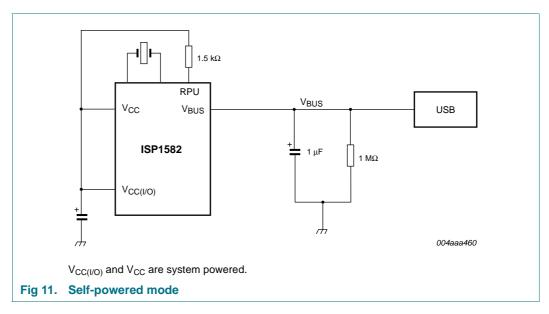
In self-powered mode,  $V_{CC}$  and  $V_{CC(I/O)}$  are supplied by the system. See Figure 11.
