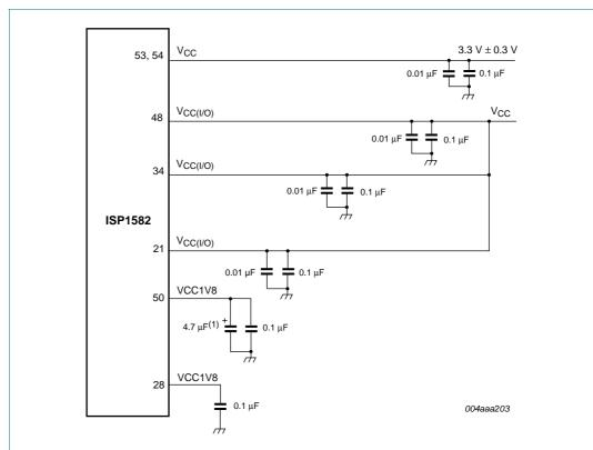
(1) At the V<sub>CC</sub> input (3.3 V) to the USB controller, if the ripple voltage is less than 20 mV, then 4.7  $\mu$ F standard electrolytic or tantalum capacitors (tested ESR up to 10  $\Omega$ ) should be OK at the VCC1V8 output. If the ripple voltage at the input is higher than 20 mV, then use 4.7  $\mu$ F LOW ESR capacitors (ESR from 0.2  $\Omega$  to 2  $\Omega$ ) at the VCC1V8 output. This is to improve the high-speed signal quality at the USB side.
