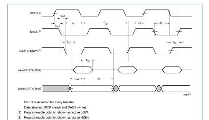
Fig 19. GDMA mode timing (bits MODE[1:0] = 01)
