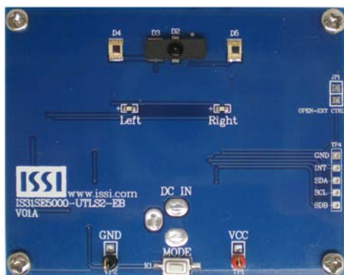
Figure 1: Photo of IS31SE5000 Evaluation Board
