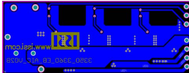
Figure 4: PCB Layout-Bottom Layer
