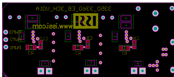
Figure 5 Component Placement Guide -Bottom Layer
