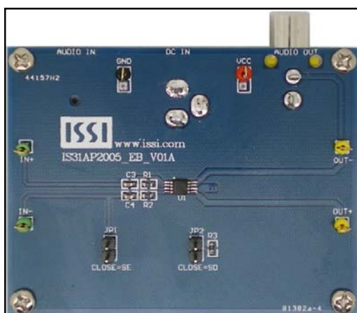
Figure 1: Photo of IS31AP2005 Evaluation Board
