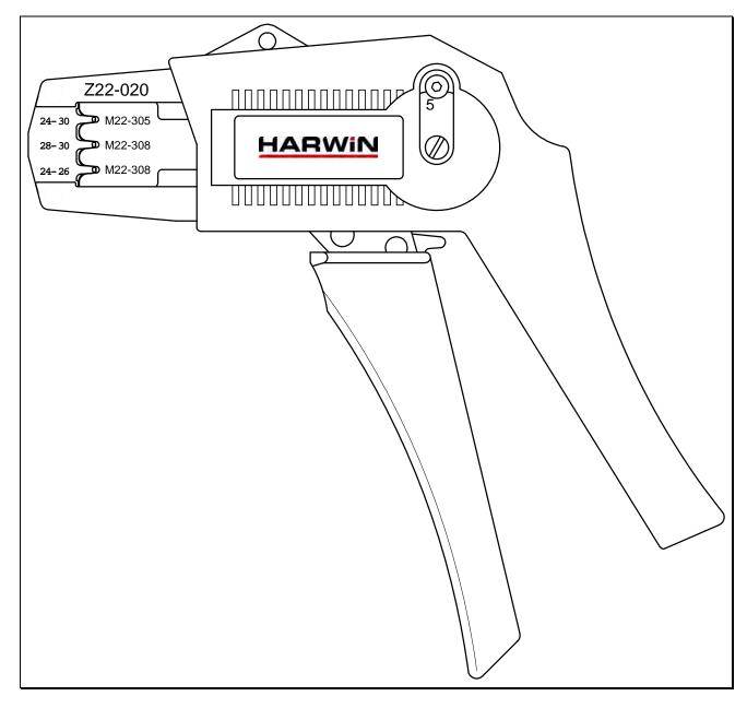
This Hand Crimp Tool has been designed for use with the following crimp contacts:
