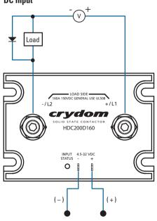
(D) Inductive loads must be diode supressed as indicated.
