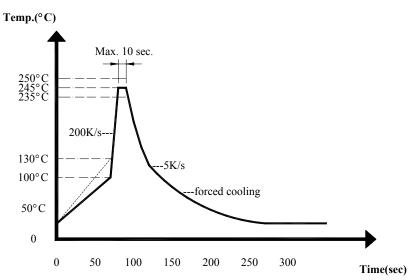
Recommendable wave soldering condition is as follows.
