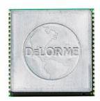
CPU of ARM7TDMI microprocessor. The end result provides excellent navigation performance in the most challenging urban environments. The DeLorme GPS2056-10 offers RTCA-SC159 / WAAS / EGNOS support and provides excellent sensitivity and high configurability in a small package.
