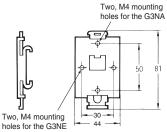
To mount the Relay to DIN Track, first mount it to the One-touch Mounting Plate and then attach it to the DIN Track as shown in the diagram.
