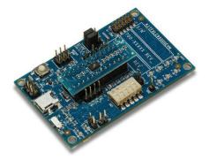
With internal flash memory, the FXLC95000CL can be re-programmed on the fly. New sensors for new applications are now possible based on programming the FXLC95000CL sensor hub with full customization for the end user and mobile device-level through software.
