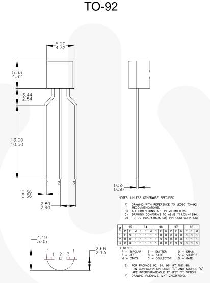
Figure 1. 3-LEAD, TO-92, MOLDED 0.200 IN LINE SPACING LD FORM (J61Z OPTION) (ACTIVE)
