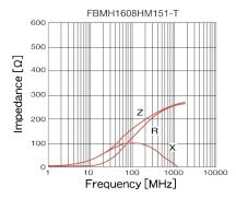
The data is reference only. Electrical characteristics vary depending on environment or measurement condition. TAIYO YUDEN reserves the right to make change to the Date at any time without notice. Before making final selection, please check product specification. 2013.10.31
