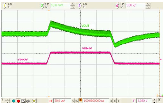
Figure 21. Line Transient, I_{LOAD}=1.0\text{ A} , t_R=t_F=10\ \mu\text{s}
