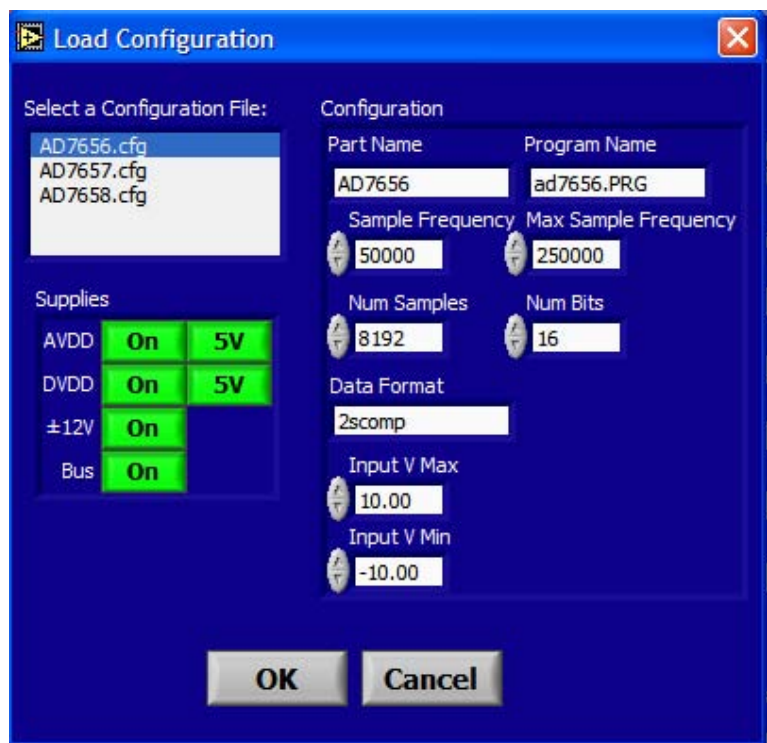
Figure 4. AD7656-1/AD7657-1/AD7658-1 Evaluation Software, Load Configuration Window
