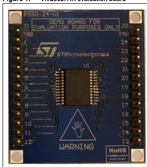
Figure 1. VNQ5027AK evaluation board
