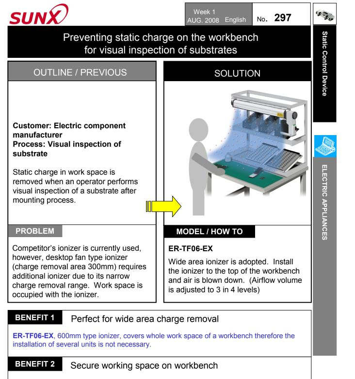
**ER-TF06-EX** can be installed overhead so that workbench will not be occupied. Air blow angle can be easily adjusted after the setup.
