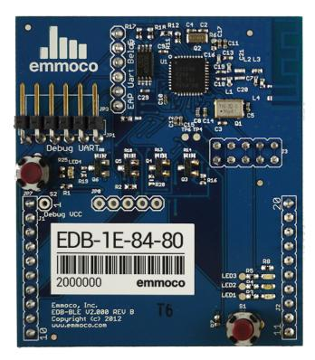
**EDB-BLE** - an easy-to-use *Bluetooth*® Smart development board that comes with unrestricticted access to the Emmoco development tools including free apps on the iTunes store. It is compatible with any microcontroller that has a serial interface or can be directly connected to the TI MSP430 LaunchPad as a Boosterpack.
