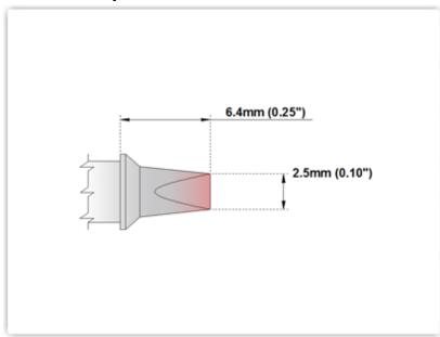
EBM7CP200 Chisel, 2.50mm (0.10"), 30°
