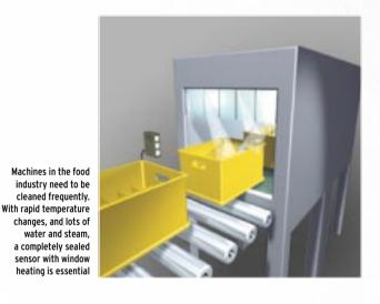
Thanks to the optic link, the sensor can be remotely set and checked while it is operating in an area where access is restricted
