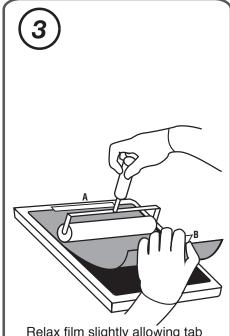
Relax film slightly allowing tab 'A' edge to come close to LCD panel, but not touch. With free hand, use roller to laminate film into place in one continuous sweep. Remove tabs 'A' and 'B'. Use plastic stylus to complete lamination along edges as necessary. Clean with acetone as necessary.
