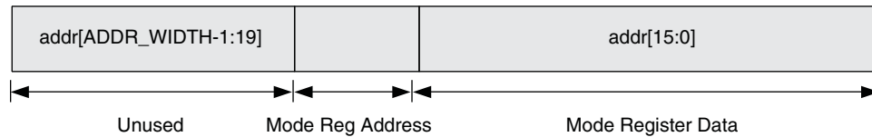
Figure 2-8. User-to-Memory Address Mapping for MR Programming
