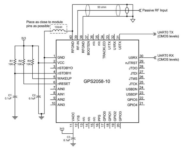
The following describes the minimum GPS2058 GPS receiver module connectivity necessary to obtain a position fix with passive antenna and host connection.
