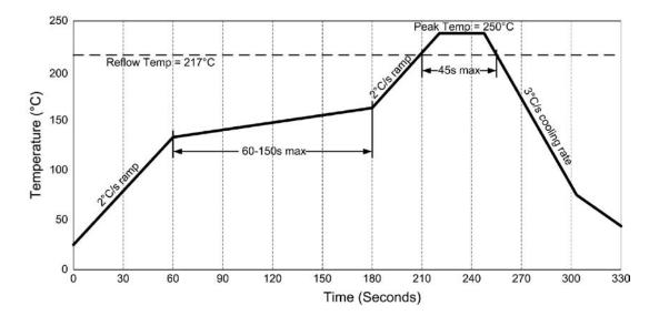
Ideally the module will only be subjected to a single reflow process with the module on the top side surface of the printed circuit board. Additional reflows may cause bridging between pads, or potential damage to the module.
