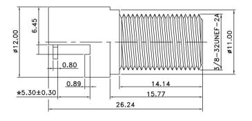
Body: Brass/Nickel Insulator: Delrin Pin: Copper/Tin \*
