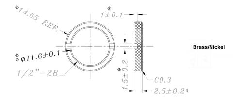
This is a basic dimensional drawing. If you require a more detailed drawing or if this connector does not fit your exact requirement please email - mailstop@bomarinterconnect.com or call 973-347-4040 for an alternate solution.
