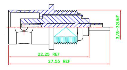
Body: Brass/Nickel Insulator: Delrin Pin: Brass/Gold
