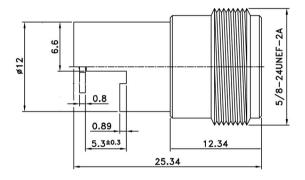
Body: Brass/Nickel Insulator: Teflon Pin: Brass/Gold
