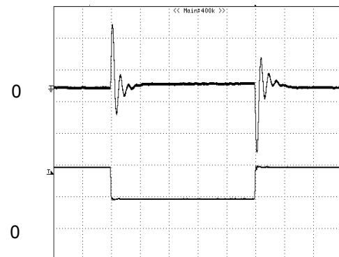
Figure 9: Output voltage response to step-change in load current (75%-50%-75% of I_{o,max} ; di/dt = 1.0A/\mu s ). Load cap: 100 \mu F tantalum capacitor and 1 \mu F ceramic capacitor. Top Trace: V_{out} (100mV/div, 200us/div), Bottom Trace: I_{out} (10A/div). Scope measurement should be made using a BNC cable (length shorter than 20 inches). Position the load between 51 mm to 76 mm (2 inches to 3 inches) from the module
