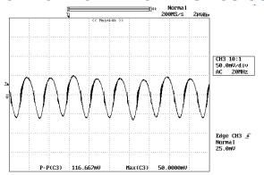
**Figure 11:** Input Terminal Ripple Current, i<sub>c</sub>, at full rated output current and nominal input voltage with 12μH source impedance and 33μF electrolytic capacitor (50mA/div, 2us/div)
