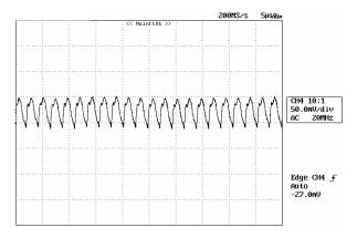
**Figure 14:** Output voltage ripple at nominal input voltage and rated load current (lo=3A) (50 mV/div, 5us/div). Load capacitance:  $1\mu$ F ceramic capacitor and  $10\mu$ F tantalum capacitor. Bandwidth: 20 MHz. Scope measurements should be made using a BNC cable (length shorter than 20 inches). Position the load between 51 mm to 76 mm (2 inches to 3 inches) from the module
