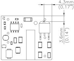
**Figure 20:** Temperature measurement location The allowed maximum hot spot temperature is defined at 127  $\mathcal{C}$ .
