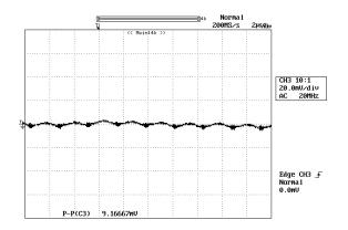
**Figure 12:** Input reflected ripple current, i<sub>s</sub>, through a 12μH source inductor at nominal input voltage and rated load current (20 mA/div, 2us/div)
