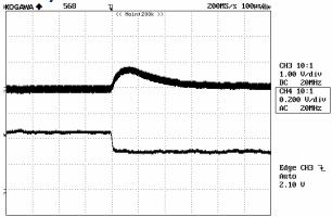
**Figure 8:** Output voltage response to step-change in load current (75%-50% of lo, max; di/dt =  $0.1A/\mu$ s). Load cap:  $10\mu$ F tantalum capacitor and  $1\mu$ F ceramic capacitor. Top Trace: Vout (200mV/div, 100us/div), Bottom Trace: lout (1A/div). Scope measurement should be made using a BNC cable (length shorter than 20 inches). Position the load between 51 mm to 76 mm (2 inches to 3 inches) from the module.
