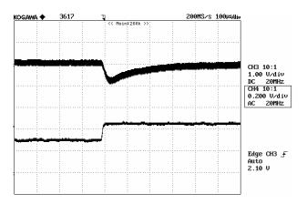
**Figure 9:** Output voltage response to step-change in load current  $(50\%-75\% \text{ of lo, } max; \text{ di/dt} = 0.1\text{A/}\mu\text{s})$ . Load cap:  $10\mu\text{F}$  tantalum capacitor and  $1\mu\text{F}$  ceramic capacitor. Top Trace: Vout (200mV/div, 100us/div), Bottom Trace: lout (1A/div). Scope measurement should be made using a BNC cable (length shorter than 20 inches). Position the load between 51 mm to 76 mm (2 inches to 3 inches) from the module.
