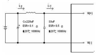
**Figure 10:** Test set-up diagram showing measurement points for Input Terminal Ripple Current and Input Reflected Ripple Current. Note: Measured input reflected-ripple current with a simulated source Inductance ( $L_{TEST}$ ) of 12  $\mu$ H. Capacitor Cs offset possible battery impedance. Measure current as shown below.
