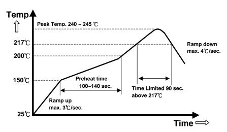
Note: The temperature refers to the pin of S36SE, measured on the pin +Vout joint.
