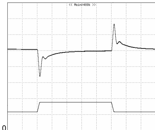
Figure 8: Output voltage response to step-change in load current (75%-50%-75% of I_o , max; di/dt = 0.1A/\mu s ). Load cap: 10\mu F , tantalum capacitor and 1\mu F ceramic capacitor. Top Trace: V_{out} (100mV/div, 200us/div), Bottom Trace: I_{out} (5A/div). Scope measurement should be made using a BNC cable (length shorter than 20 inches). Position the load between 51 mm to 76 mm (2 inches to 3 inches) from the module..
