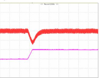
**Figure 9:** Output voltage response to step-change in load current (25%-50% of lo, max; di/dt = 0.1A/µs). Load cap: 10µF, tantalum capacitor and 1µF ceramic capacitor. Top Trace: Vout (100mV/div, 10us/div), Bottom Trace: I out (5A/div).
