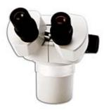
The DSZ-70 Series body can be mounted on a variety of boom stands. You choose the rack & pinion focus mount, illumination, and accessories to meet your specific requirements. Various eyepieces & auxiliary lenses can be used for desired magnification and working distance.
