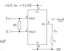
Measuring a single ended input voltage referenced to a split supply, i.e. the input voltage and the meter's power supply share the same OV rail. Ensure solder link LCOM is open.
