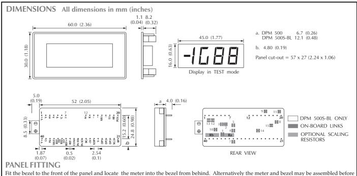
fitting to the front of the panel but care must be taken not to use excessive force. Finally fit the window into the front of the bezel.
