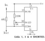
Measuring 4-20mA to read 0-999 (supply must be isolated).
