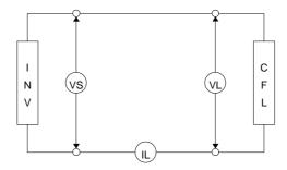
**CFL Testing Circuit**
