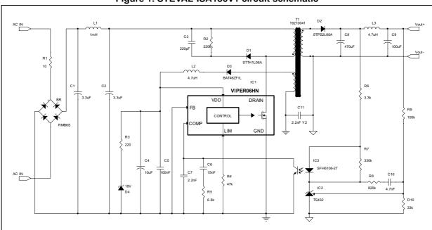
Figure 1. STEVAL-ISA136V1 circuit schematic
