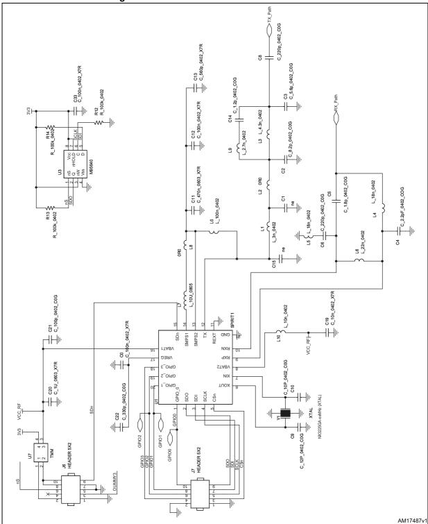
Figure 1. STEVAL-IKR001V8D circuit schematic
