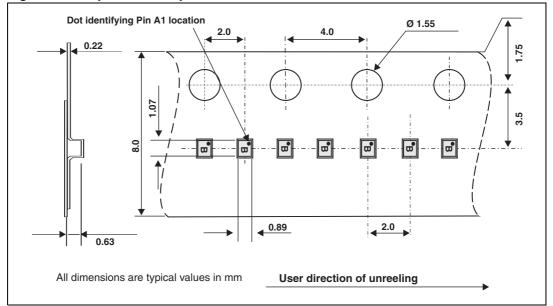
Figure 15. Tape and reel specifications
