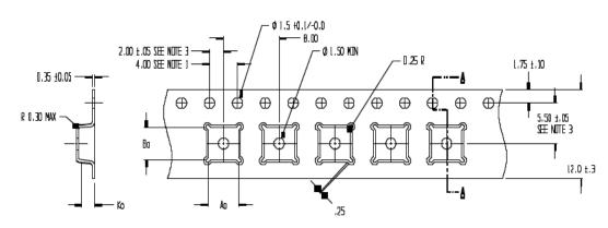
NOTES: 1, 10 SPROCKET HOLE PITCH CLMULATIVE TOLERANCE ±0.2
