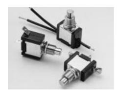
The P-Series pushbutton switches are heavy-duty, single pole switches. They are alternate action, available in single and double throw construction, with ratings up to 20 amps. Both plunger and bushing are made of plated brass. Typical actuation force is 3-5 lbs.
