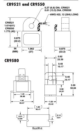
The **CR9500** Series Current Sensors provides a cost effective method for monitoring electrical current. The sensor generates a 0-5 VDC signal proportional to the input AC current. The output signal is average sensing, calibrated to RMS.
