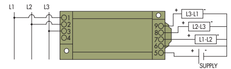
CR4860 3 Element, 3 Wire - 4-20 mA DC Output
