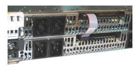
**Notes:** Shelf addressing, 8V\_INT, and current share are referenced to the most negative power output Vout(-) of the shelf. For paralleled shelves the Vout(-) terminations must be tied together in order to ensure proper operation of these functions. Modules could get damaged if this connection is not made.
