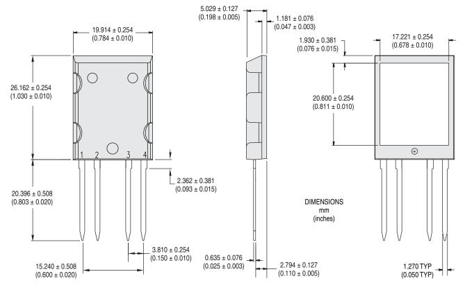
NOTE: Back-side heat sink meets 2500V<sub>me</sub> isolation to the pins.
