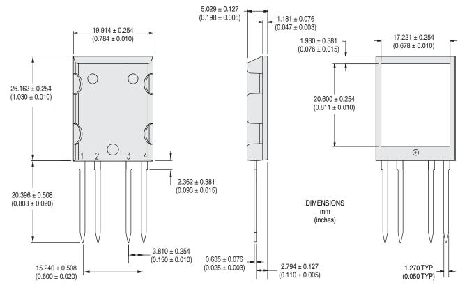
NOTE: Back-side heat sink meets 2500V<sub>rms</sub> isolation to the pins.
