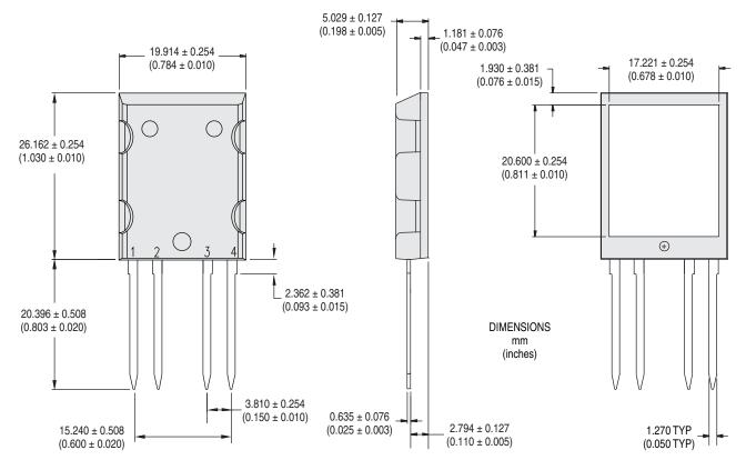
NOTE: Back-side heat sink meets  $\mathrm{2500V}_{\mathrm{rms}}$  isolation to the pins.
